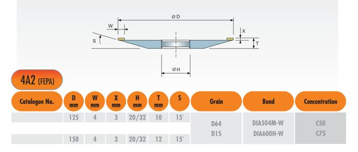
For the preparatory (rough) <u>wet</u> grinding of the cutting face of the tungsten carbide knives, it is recommended to use the bond type **DIA504M-W** and the grain size D64.
