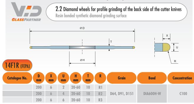
For <u>wet</u> profile grinding of the ridge of the cutter the bond type **DIA600H-W(A)** using emulsion as the coolant is recommended, for example at production of the saw blade with the grinding depth of t=0.8mm and the grit D151, or at smooth grinding with the grinding depth of t=0.05mm and the grit D64.
