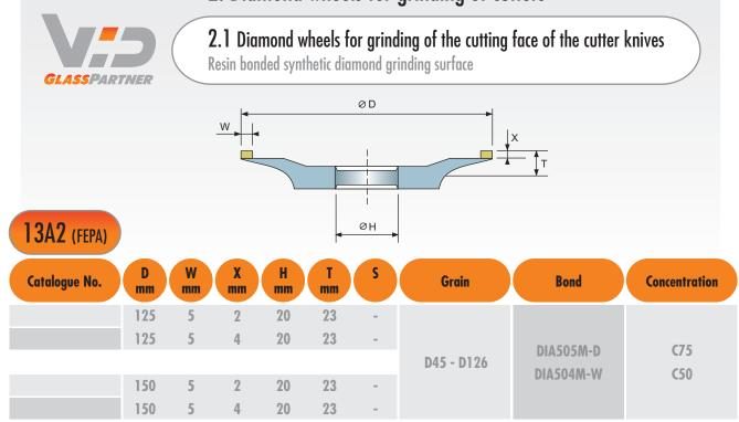
A larger width of grinding (e.g. 25mm and more) is characteristic for grinding of the cutting faces of the cutters on universal lathes. This brings a considerable reduction to the grinding regimes (e.g. grinding depth = t), as opposed to grinding of narrow surfaces (e.g. the ridge of the cutter, see 2.3). For this operation the bond types DIA505H-D(C) for dry grinding and the bond type DIA504M-W(A) for wet grinding using emulsion as the coolant are recommended.
